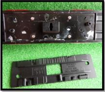
Part 3 First remove the black 3 screws that hold the body to the floor 1 at the front and 2 at the back when the body is removed take out the 4 silver screws and you will have 6 parts 2x bogies 1x under fame 1x body 1x seat unit and a floor this should take about 5 minuets
