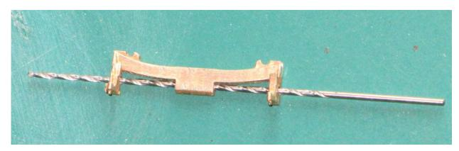
Take a long 1.5mm drill and drill through the axle bearings in the front axle support as shown. Go slowly, use plenty of lubricant and take care.
