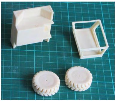
Remove any moulding pips and flash from the resin and WM castings.
