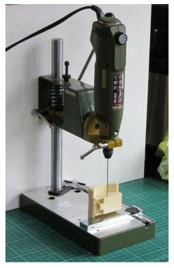
Using a long 1.6mm drill bit, drill vertically through the two dimples in the cockpit to produce the hole for the rear axle.
