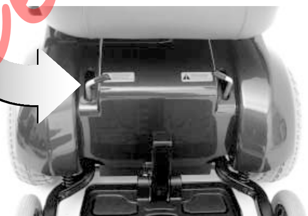
Figure 7. Drive Motors Disengaged (Freewheel Mode)
