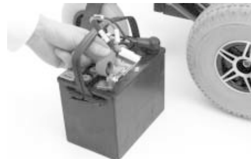
Figure 23. Connecting Wires To The Battery Terminal
