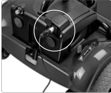
Battery Charging Socket
