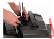
2. Turn the handle to release the battery pack, then lift out the battery pack from the main body of the scooter.
