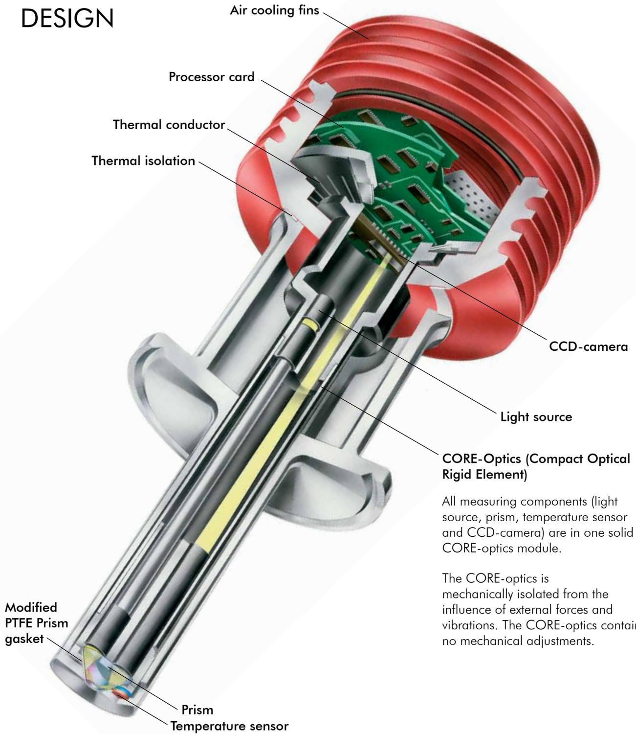
All measuring components (light source, prism, temperature sensor and CCD-camera) are in one solid CORE-optics module.
