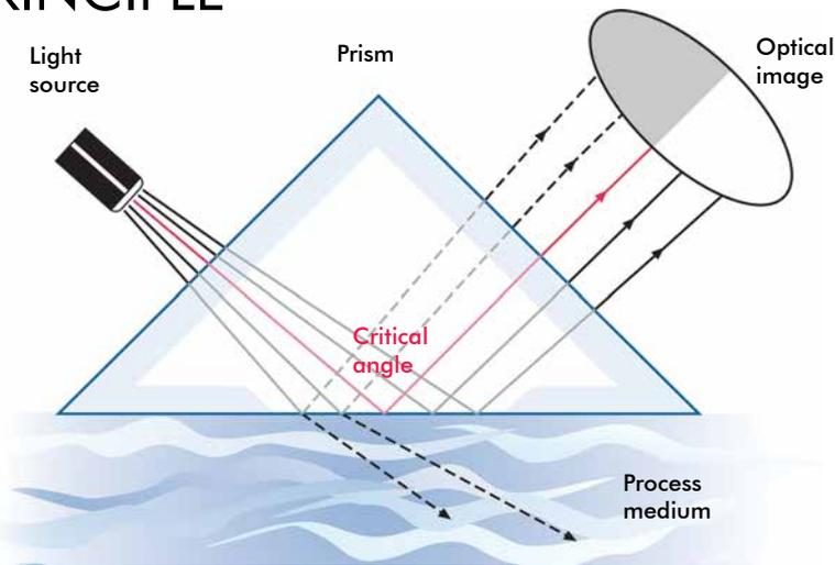
The light source emits light at the interface, between a prism and the process solution, where the rays meet the surface at different angles.
