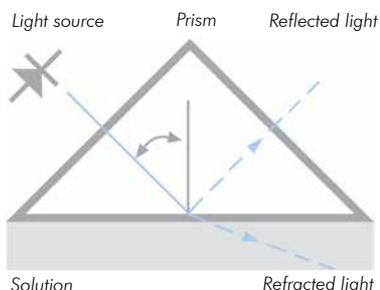
Depending on the angle, some rays undergo a total internal reflection. The rest of the light is refracted into the process solution.
