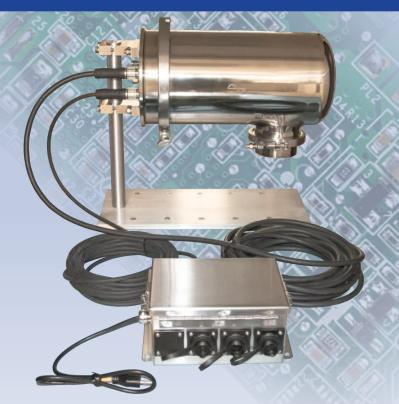
The NIR-6300 Harsh Environment Analyzer is the first choice for manufacturing environments hostile to precision instruments. Its #316 stainless-steel enclosure features IP67/NEMA 4x protection ratings that protects during rigorous wash-downs and even immersion.
