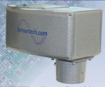
The NIR-6000 provides an on-line, real-time moisture analysis of your product. This ongoing monitoring enables forward thinking and determination of optimum drying process conditions essential for manufacturing. Our sensor employs near infrared reflectance (NIR) technology, which is continuous, non-contact and nondestructive. Your process is never impeded and your product never compromised.
