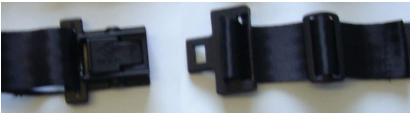
Sliplock slide added to prevent slippage
