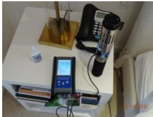
Measuring and monitoring Volatile Organic Compounds in a customer's bedroom
