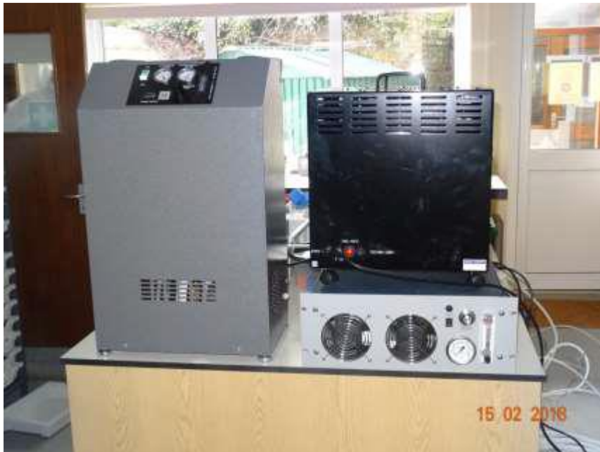
Ozone generators at 800ppm using nitrogen free air to sanitise air and some surfaces
