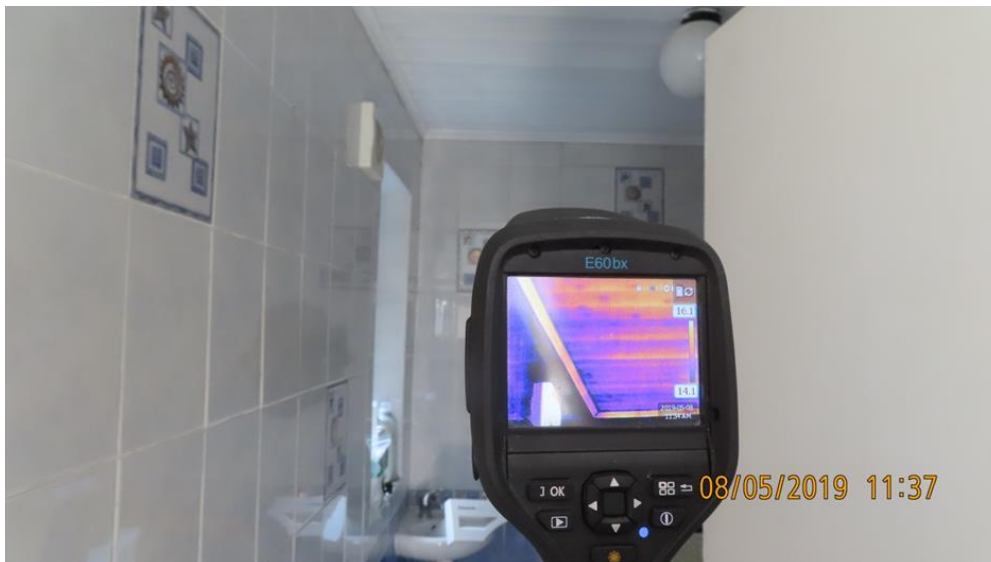
This bathroom has poor ceiling insulation and dew point condensation within ceiling cavity causing mould growth and poor health for occupants
