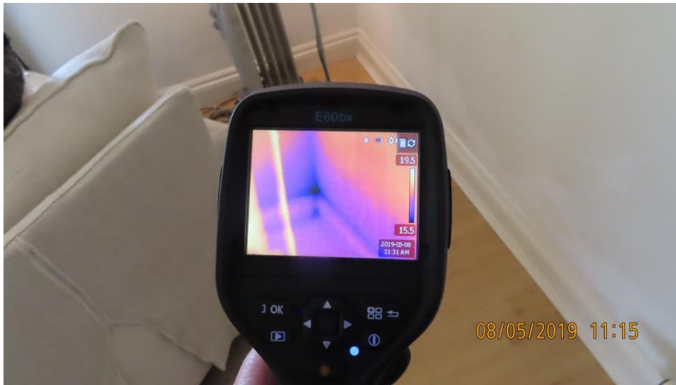
Rising damp issues caused by DIY actions
