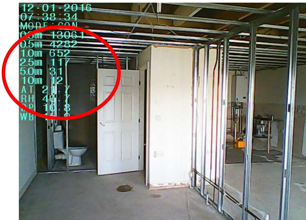
47 Monitoring dust (including mold fragments) post decontamination to assess efficacy of air cleaning
