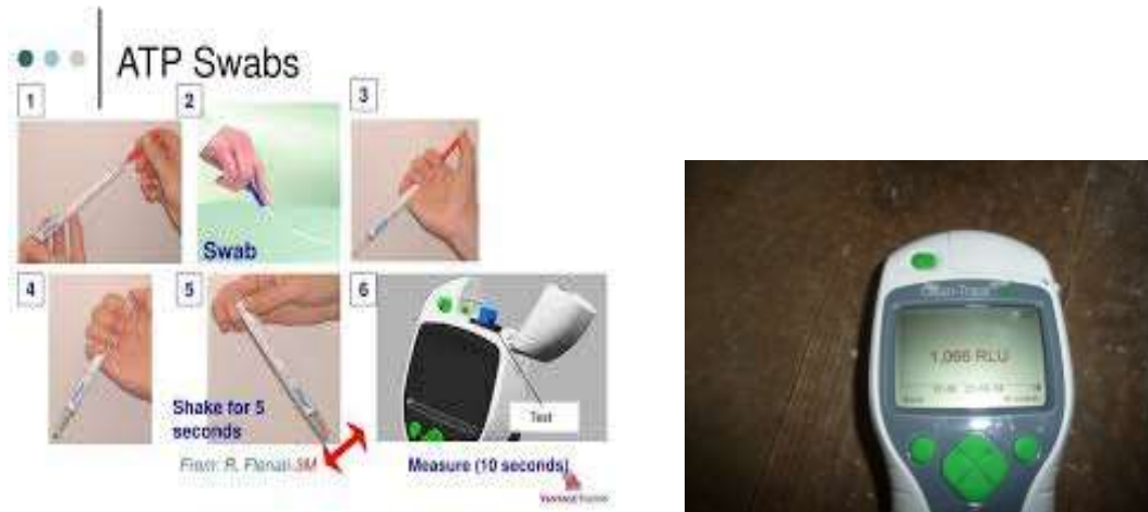
Fig 2 Showing the ATP sampling process and analysis meter
