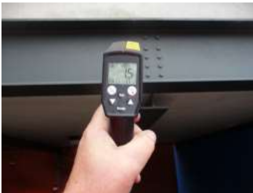
27 The temperature of the support steel 15c with lower attached steel at 0.2c acting as a heat sink
