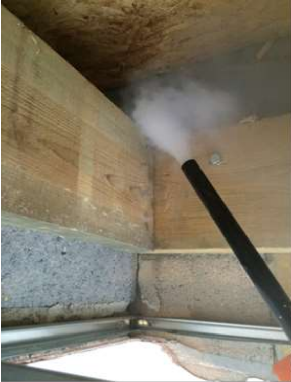
46 A smoke generator used to identify air pressure differentials and air pathways
