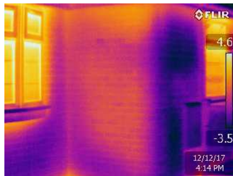
16 IR photos shows temperature range of cavity wall from -3.5 to 4.6c
