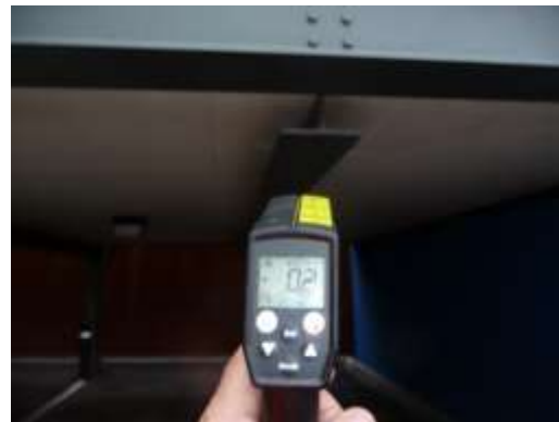
27 The temperature of the support steel 15c with lower attached steel at 0.2c acting as a heat sink
