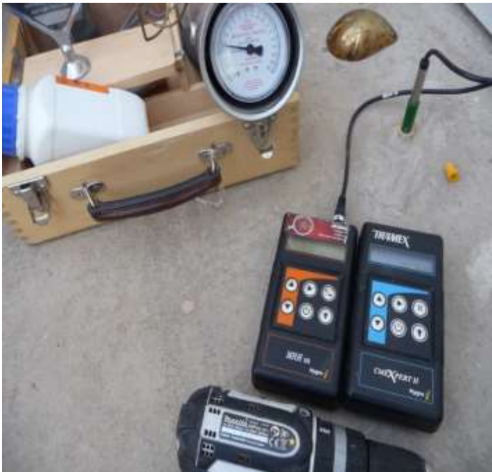
14 This shows methodology of measuring EMC and ERH in concrete floors
