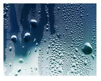
Occasionally you may get condensation forming on the external pane of glass. This is usually visible on cold, clear mornings for instance in frosty weather. This phenomenon occurs because modern glass coatings and gas filled cavities have become so efficient at keeping the heat inside the room that warmth is not able transfer to the external pane to heat it up. This is not a product fault and as the daytime temperature rises the external condensation will disappear.
