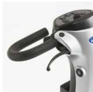
Hand brake Ensures immediate braking if required.
