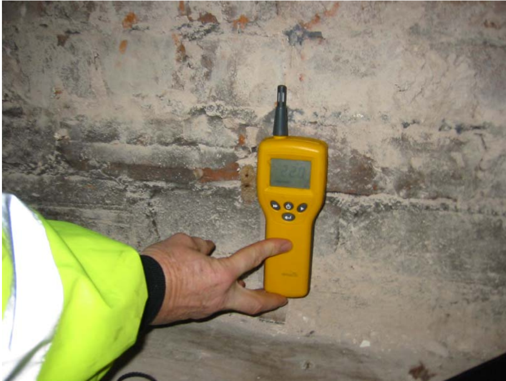
22% wme wood moisture equivalent = approximately 6% moisture content
