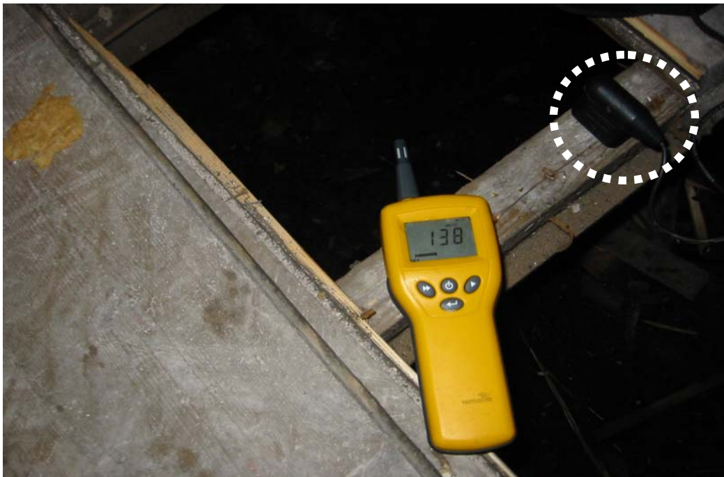
Joists at 13.8% Using penetrative spikes. Acceptably Dry without drying!
